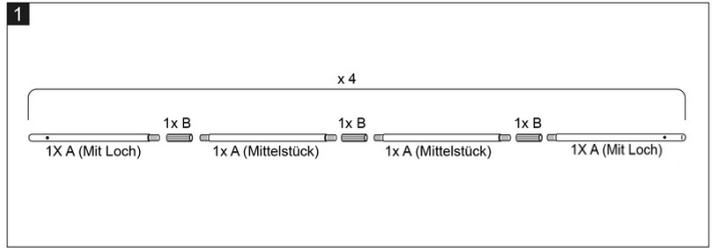
Carefully insert these 4 tent poles into the tunnels of the tent fabric C and set up the teepee. The protective caps E can already be attached to the feet.
